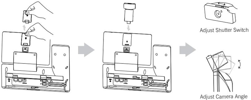
Note: The camera can only be connected to the USB port on the top of the phone. And the IP phone only supports the Yealink original USB camera CAM50.
