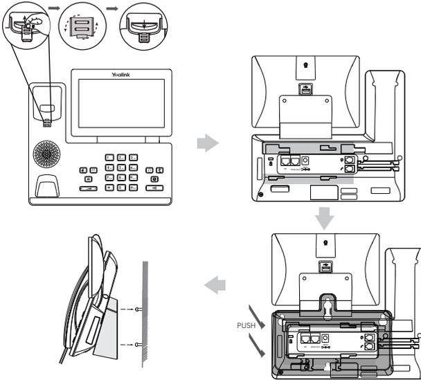
Note: The reversible tab has a lip which allows the handset to stay on-hook when the IP phone is mounted vertically. For more information, refer to Yealink Wall Mount Quick Installation Guide for Yealink IP Phones.
