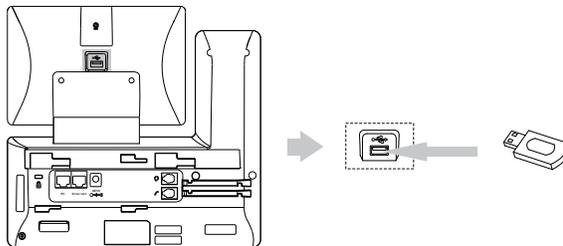
Note: The USB port (on the rear of the phone) can also be used to connect color-screen expansion module EXP50, USB headset or DECT USB dongle DD10K. For more information on how to use EXP50, refer to Yealink EXP50 User Guide. For more information on how to use USB headset, refer to the documentation from the manufacturer. For more information on how to use DD10K, refer to Yealink Smart Business Phones User Guide.
