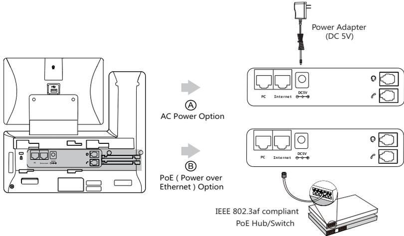
Note: The IP phone should be used with Yealink original power adapter (5V/2A) only. The use of the third-party power adapter may cause the damage to the phone.
